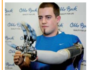
The world's first fully thought-controlled prosthesis by Otto Bock Vienna, Vienna's General Hospital and the Medical University of Vienna.
