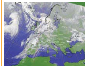
Gepard: Polar-stereographic projection of the European region; IR (infra-red) cloud image together with a land/sea background, geographical net and the major European cities drawn as overlay.
