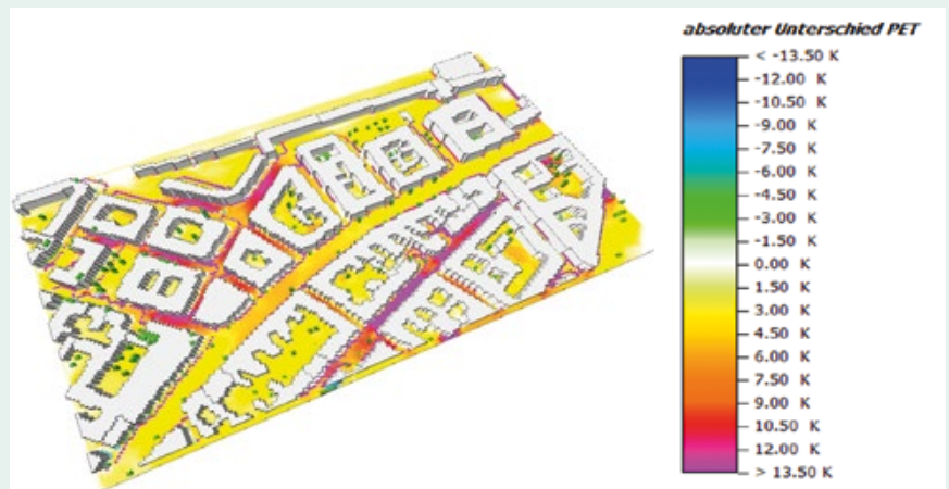
ENVI-met model of differences in perceived temperature [PET] comparing greened and un-greened Mariahilferstraße (Source: Bernhard Scharf, BOKU)
