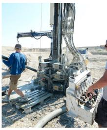
Step 4: On the right is the control console, which is used to operate the drilling rig manually. Up to two heat exchangers can be inserted into the ground in one day.
