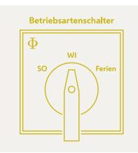
A simple switch: This switch allows even laypeople to operate the HVAC system safely and easily, switching between winter, summer and holiday mode. This saves energy and costs. The primary school in Krottenbachstraße in the 19<sup>th</sup> district, for example, was equipped with this switch, ensuring energy-efficient operation.
